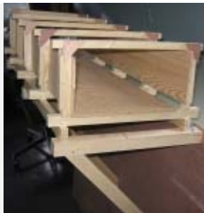
A 1/8 scale model of the Hanging Flume, built by Vertical Access.
